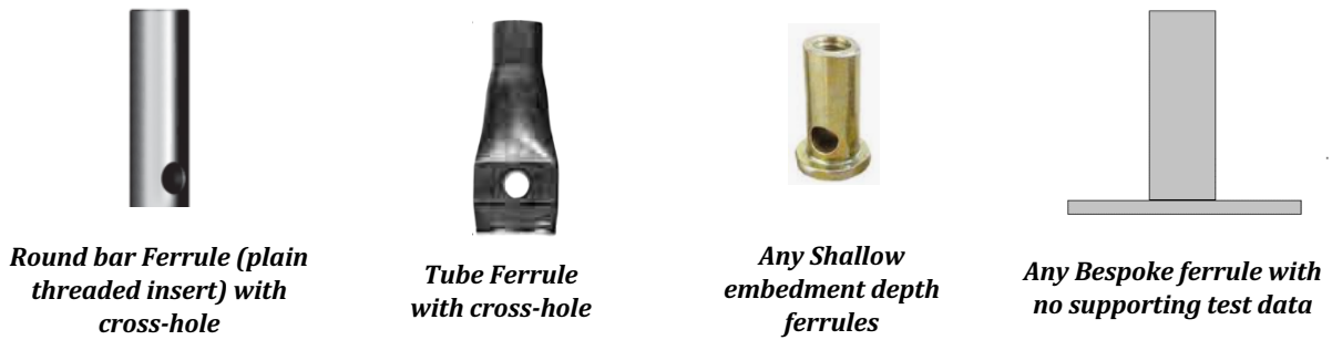
Figure 8: Examples of non-compliant systems.
