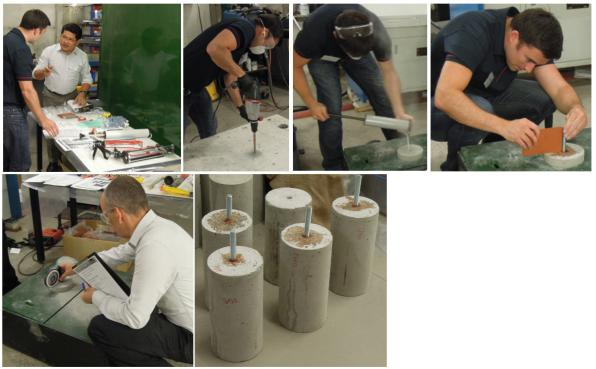
Figure 2: Vertical down bonded anchor installation
